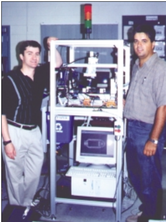
Project director, Dr. Gary Bone (left) and Ph.D. student Lucian Bulan (right), with the machine vision inspection system they developed for Sandco Automotive. The unit inspects approximately 250,000 parts per week.
