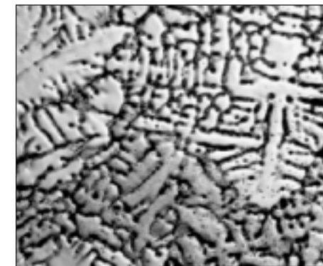
Optical Micrographs of cast aluminum wrought alloy samples. Image at left is from a conventional cast sample showing dendrites of primary aluminum and image at right is from a sample cast using CDS method showing globular/non-dendritic primary aluminum phase.
