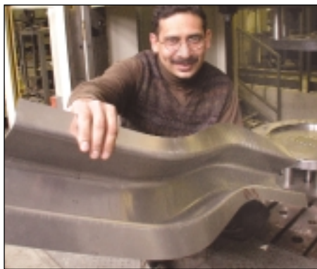
Dr. Mukesh Jain holds an aluminum S-Rail, which has undergone bending and twisting in the lab's new press.
